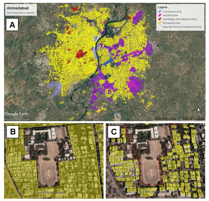
Figure 4: The research team utilized Google Earth satellite imagery and city maps to estimate the extent of residential zones (panels A and B) and available residential roof area (panel C) in Ahmedabad to understand the energy savings benefits of cool roofs (Credit: Joshi et al., 2022).<sup>6</sup>
