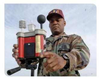
Figure 2.2: Measurement of the parameters comprising the Wet-Bulb Globe Temperature (WBGT) Index by military personnel. From left to right, the sensors are the dry-bulb thermometer ( $T_{db}$ ), natural wet-bulb ( $T_{wb}$ ) and the globe thermometer (T<sub>g</sub>), which are incorporated by algorithm to represent the WGBT.
